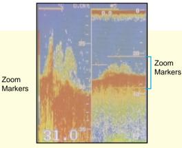
The zoom markers follow the bottom contour automatically giving us an expanded view of the area near the bottom. This is done even under conditions of changing depth.
